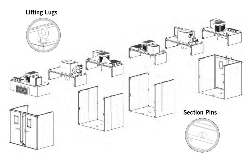
**Gruenberg Steri-Dry Sterilizers** are designed and constructed in modules, sized for ease of rigging and assembly without modification of the existing facility. This design flexibility ensures that the project costs are well contained.
